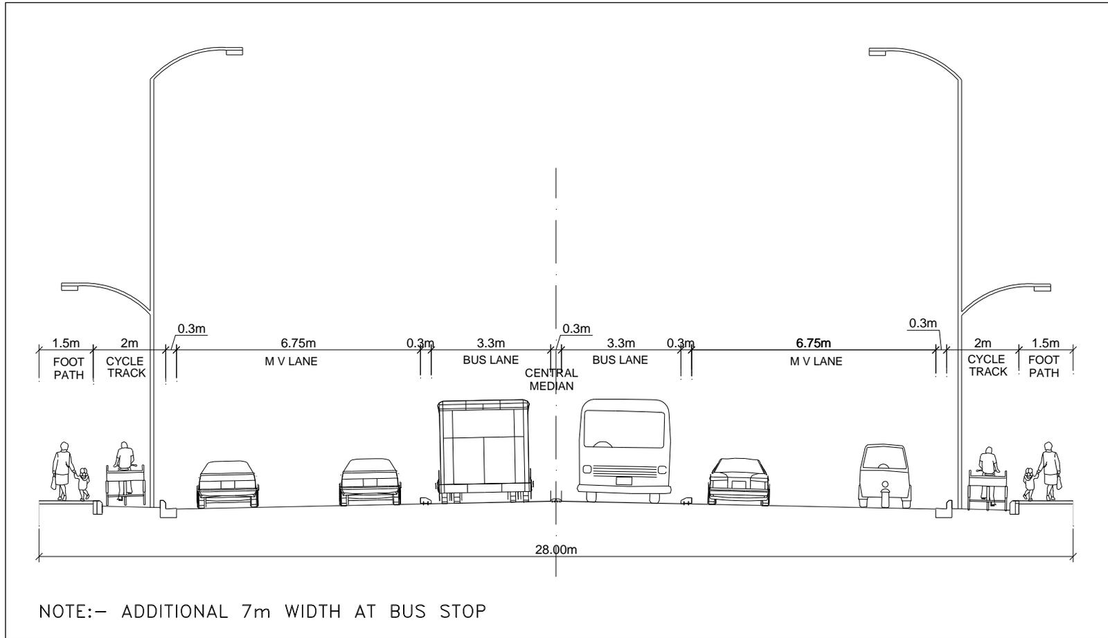
**Figure 6.9 Typical Cross-Sections of Road with Elevated LRT and Monorail**
