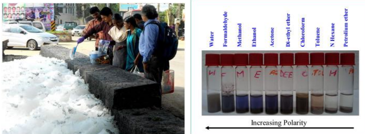
Fig. 6.3.1 and 6.3.2: Collection of foam sample from Varthur lake and analysis of elution of the liquid phase of the foam in different solvents in the order of increasing polarity
